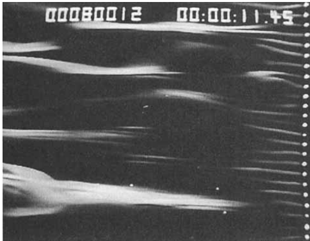
FIGURE 10. A typical sequence of the burst event visualized with the smoke-wire technique with a sheet of laser light. Flow is from right to left.
